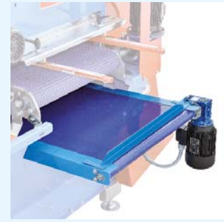
53 Belt for the recycling of the exceeding soil.
