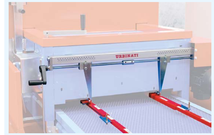
54 Rapid adjustment with handles of tray guide width.
